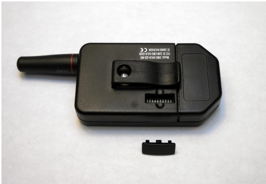
Hand-held Transmitter showing code setting switch access door removed
